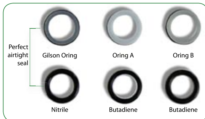
Figure 3: The level of elasticity based on the ASTM test method is 80 shores for the PIPETMAN® O-ring compared to only 70 shores for the counterfeit ones. When the hardness of the seal is increased, its resistance to deformation is also increased resulting in cracks.
